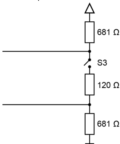
Fig. 21: RS 485 switchable terminating resistor
