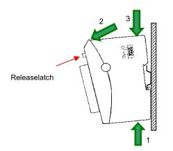
Fig.: 11 Disassembling the B-Nimis MC-Pi & BC-Pi
