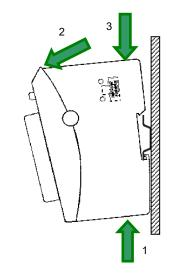
Fig.: 4 Disconnecting the B-Nimis MC-Pi & BC-Pi
