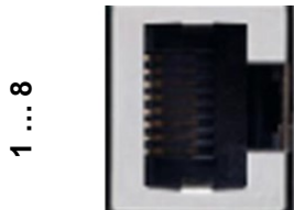
Fig.: 88 CAN interface on X16
