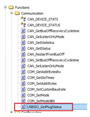
The example below shows a function block in CODESYS that checks the state of all 4 maximum possible USB serial interfaces and returns the first USBCOM Port interface found. If no interface is found, the function reports -1. The default COM Port for USBSIO devices starts at COM10 to COM13.
