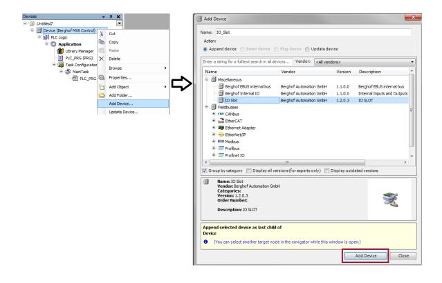
In the "Add device" window, you now have a categorized overview of all the devices that you can connect to the controller. Among them, all of the fieldbus masters installed in CODESYS V3 and their slaves and the devices for the integrated I/Os.
