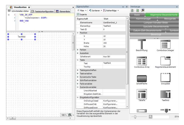
In contrast to the normal editor window (for programs, modules and functions), the visualization editor has additional sub-windows. The largest part of the window is the visualization editor itself (dotted background), which displays the visualization with all its elements. Above this editor window, there are three windows cumulated in a group of tabs:
