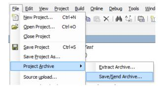
A new window opens in which you can now select which additional objects are to be loaded into the project archive. For an error-free translation of the project, after opening the archive, it is recommended to select at least all referenced objects.
