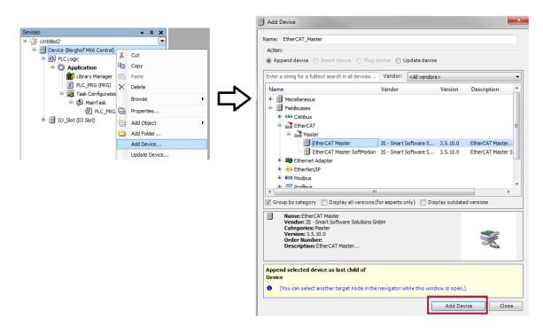
In the "Add device", you now have a categorized overview of all devices which you can connect to the controller. Including all of the fieldbus masters installed in CODESYS V3 and their slaves and the devices for the integrated I/Os.
