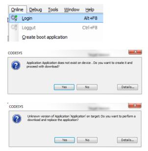
In all cases, confirm with **"yes"**. The only exception would be if the message comes that there are still errors in the program. In this case, cancel the log in and first find the errors in the program and rectify them. CODESYS V3 then starts to load the application onto the controller.
