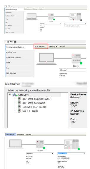
Alternatively, you can also scan directly to a controller, if the IP address is known, just type in the IP address of the controller in the text box below the controller symbol and start the scan with the Enter key.
