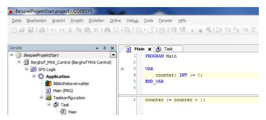
For the program to be called, an object of the type "Task configuration" must be inserted. This object automatically creates a sub-object of type "Task". You can configure this by double-clicking on the "Task" object. Select "Add call" and then select your already created "Program" object.
