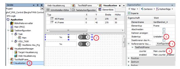
Edit the "Visualization" visualization (1) and insert a visualization element "Frame" from the "Basic" category in the "Tools" window. Then select the frame (2) and go to the "Properties" window. Next, search for the "Referenced Visualizations" property and open the dialog for referencing the visualizations with a mouse click on the "Configure..." button(3).
